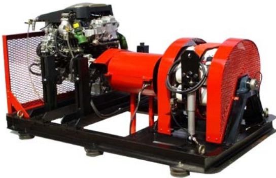
Test bed with air cooled eddy current absorber
