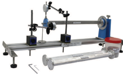
ST316 Unsymmetrical Cantilever
